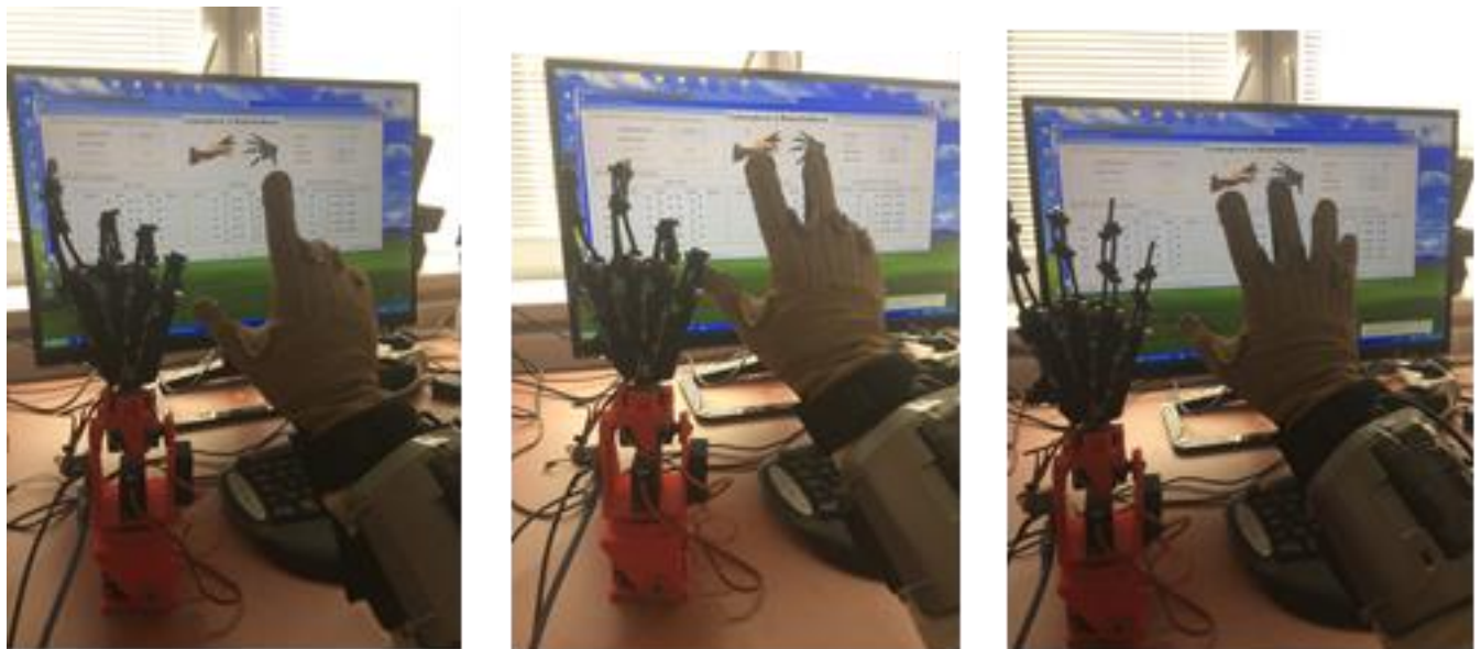
Figure 6. Experimental verification of robotic hand movements
